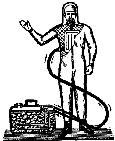
Figure 9. Extraction Principle: Rescue workers carried backpacks containing cooling devices; now these devices are placed in a separate container.
